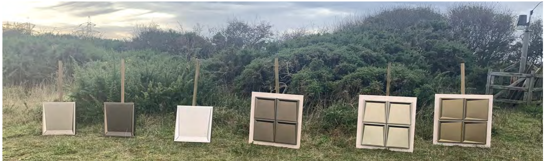
Figure 7.36: The range of scaled panels reviewed within the Sizewell context for turbine hall facades
